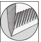
Figure 11b. Retention of larger microflutes adjacent to edge helps when cutting fiberous foods.
