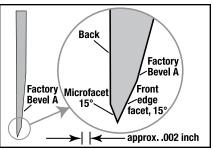
Figure 10d. Cross-section of a typical factory traditional Asian knife edge, magnified 50x (right-handed).
