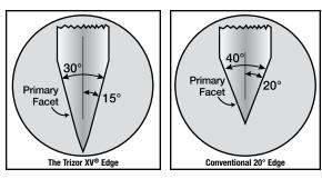
Figure 1. The Trizor® XV Edge is sharper with the added durability of the triple bevel edge.
