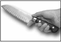
Figure 14. If your blade has a significant choil it may be helpful to place our finger behind it as shown when sharpening.
